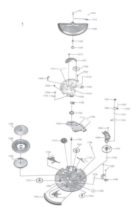
1000 Plate 1002 3/4 plate bridge 1005 Pallet cock 1026 Rotor 1030 Balance cock 1031 Bridge for automatic device 1040 Stem cock 1046 Rotor support 1100 Ratchet wheel 1101 Crown wheel 1104 Clicking spring
